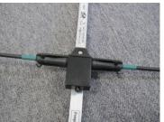
Once you have screwed both driver elements to the box, tighten up the cable ties for extra security (but not too tightly). If you are planning to disassemble the antenna you may wish to keep the tie undone or purchase additional cable ties.
