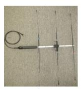
The Cable is normally delivered attached to the Antenna. However, if it is not attached or needs to be replaced, then holding the Yagi handle, carefully screw the TNC connector of the cable (next to the rubber shroud) into the female TNC socket fitted in the handle end until finger tight. Carefully push up the shroud over the end of the handle (Do not pull down on the antenna cable).
